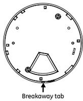
If the head must lock to the base, break away the locking tab shown below using a pair of pliers.
