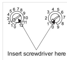
**Example:** device address 21, set TENS rotary switch to 2 and set the ONES rotary switch to 1.
